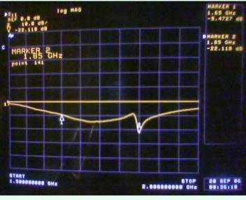
S11 plot of open-ended circular waveguide antenna prototype
