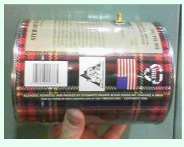
Coffee can 1.5–2.0GHz as open-ended circular waveguide antenna—female SMA attached to ¼ wavelength probe for TE mode excitation
