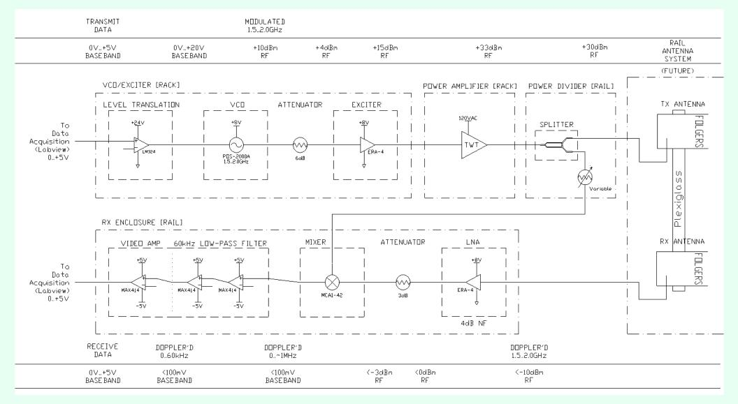
Coffee Can Radar Block Diagram
