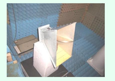
500MHz..6GHz Anechoic Range Antenna for reference testing
