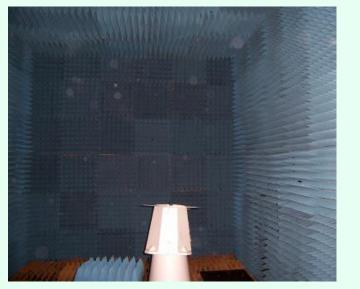
Anechoic chamber rotary antenna-under-test location
